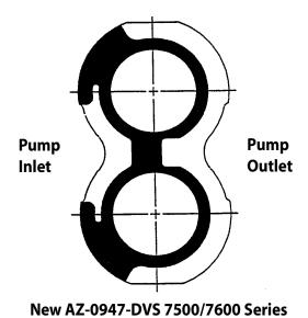
Our AZ-0947-DV 7500/7600 series thrust plate used in dry valve applications, has been superseded. Please now use thrust plate AZ-0947-DVS for all future dry valve pump needs.
