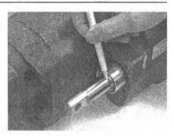
**6.** Apply light coating of grease to small O-ring and carefully place it into large detent groove in valve spool.
