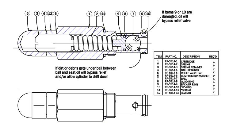
\* In the event the relief valve is disassembled - Calibration must be done on a test stand To set relief valve to 2500 PSI, when it is set at 2000 PSI from the factory remove item #5, loosen item #12, turn item #3 3/8 of a turn clockwise then tighten item #12 and replace item #5.
