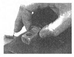
**2.** Remove retaining ring from valve spool.
