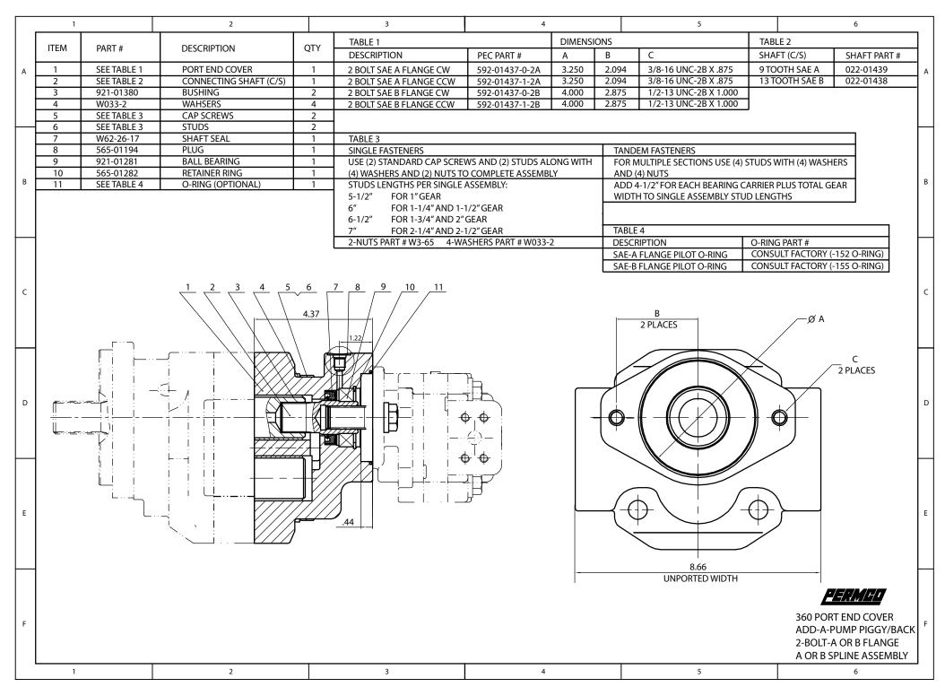
124 SERIES BUSHINGS DO NOT HAVE LUBE GROOVES; BUSHINGS ARE INSERTED WITH BUTT JOINTS AT 12:00 O-CLOCK AND 6:00 O-CLOCK USE PART NUMBER T-1194 ASSEMBLY FOR PROPER BUSHING INSTALLATION
