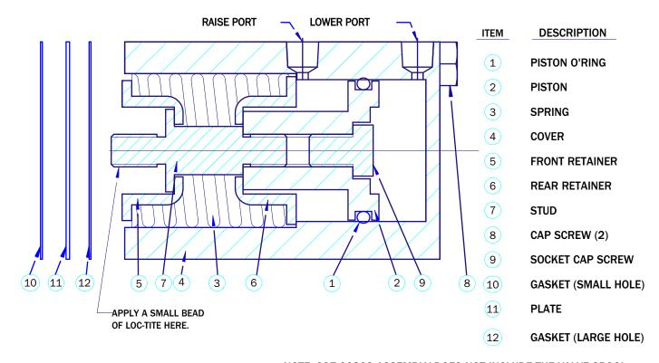
NOTE: 997-00863 ASSEMBLY DOES NOT INCLUDE THE VALVE SPOOL.
