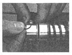
**8.** Apply a light coating of grease to quad seal ring. Slip snap ring onto clevis pin to secure it.
