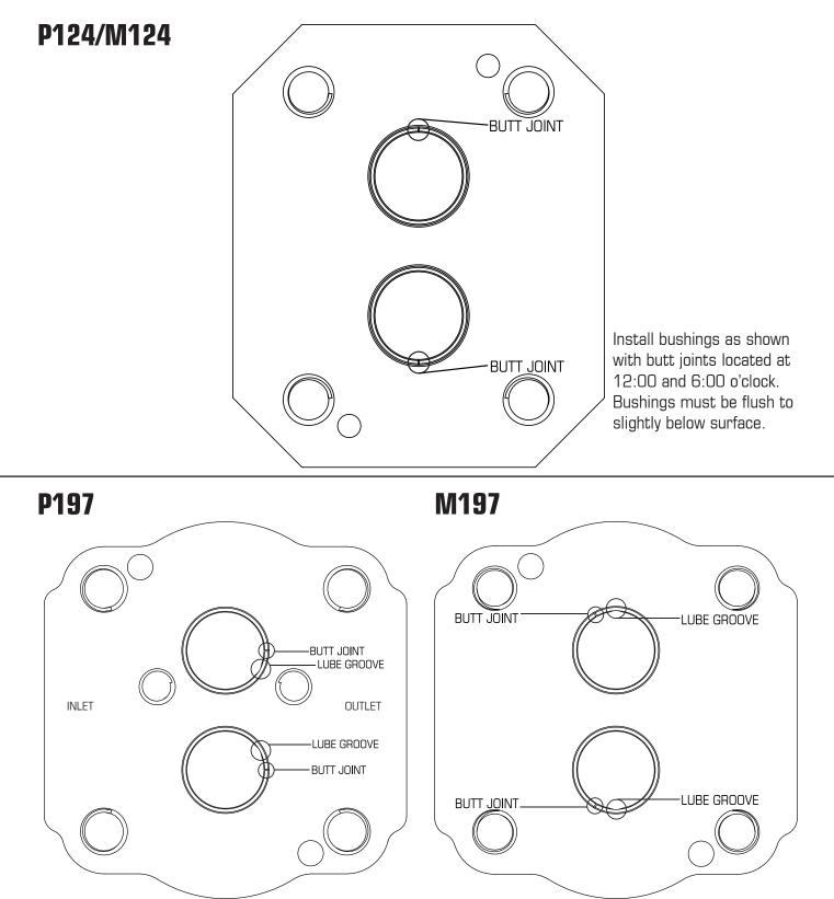
Install P197 series bushings with lube grooves and butt joints as shown for optimum performance. However, bushings may alternately be installed per M197 diagram and must be flush to slightly below the surface.
