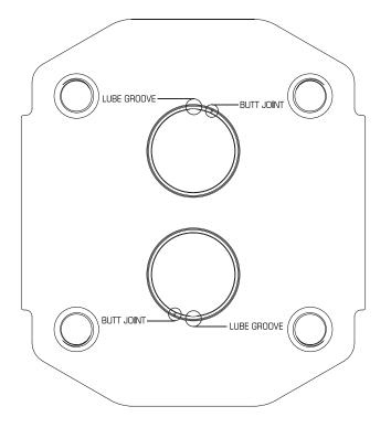
Install bushings as shown with lube grooves at 12:00 and 6:00 o'clock. Bushing OD chamfer/ lead-in is down and square corner must be flush to slightly below surface.
