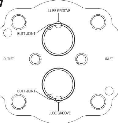
Install bushings with lube grooves and butt joints as shown. Bushings must be flush to slightly below the surface.
