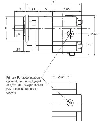
Suction Port side location, available in 7/8", 1" or 1-1/4" SAE Straight Thread (ODT), Metric Straight Thread, BSPP, SAE Split Flange or Metric Split Flange
